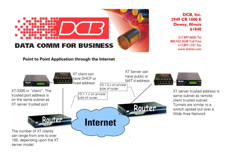
Telex IP addresses: 192.168.2.x at both ends of the link.
